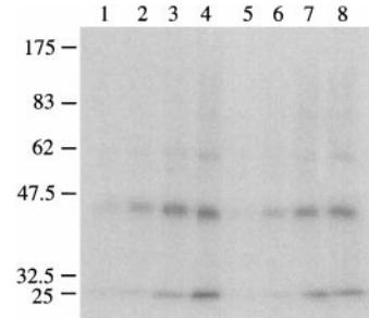
**FIG. 3.** Concentration and Mg<sup>2+</sup> dependence of photoaffinity labeling of Kir6.2 with [<sup>32</sup>P]ATP-AA. Membrane proteins (20 μg) from COS-7 cells expressing Flag-Kir6.2 were photoaffinity-labeled with 10 μM (lanes 1, 5), 20 μM (lanes 2, 6), 50 μM (lanes 3, 7), or 100 μM (lanes 4, 8) [<sup>32</sup>P]ATP-AA in the absence (lanes 1–4) or presence (lanes 5–8) of Mg<sup>2+</sup>.
